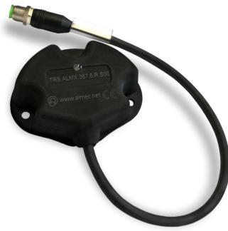
The TRS.ALMX is an inclinometer sensor based on a double CPU, a double 3D-MEMS accelerometer and a double gyroscope, in a fully redundant circuit scheme, with 2 independent CAN-Bus lines.
