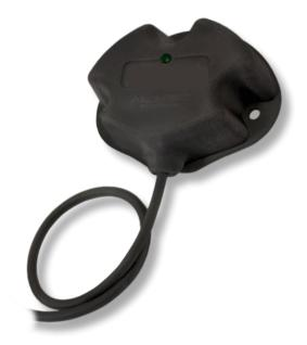
The TRS.ALMX is an inclinometer sensor based double CPU, a double 3D-MEMS accelerometer and a double gyroscope, in a fully redundant circuit scheme, with 2 independent CAN-Bus lines.
